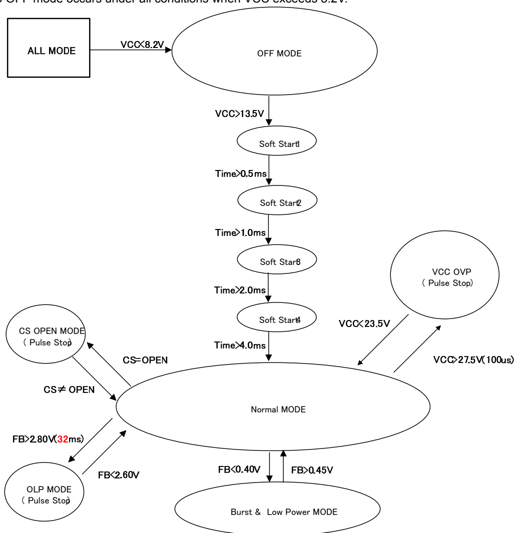
Figure 29. Sequence Diagram (BM1Pxx1 Series)
