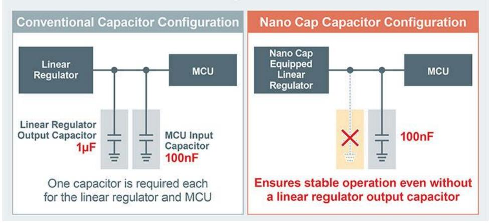
Eliminating the output capacitor solves capacitance issues in a variety of applications
