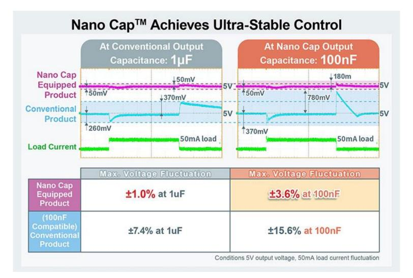
Achieves ultra-stable operation with a voltage fluctuation of +± 5% even with 1/10th the capacitance
